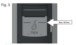
If you require a lower rate of heat effect, fill the combustion chamber with less wood. Allow lower combustion airflow. Do not forget that the combustion airflow must never be completely closed when lighting up. It is important to maintain the layer of embers. Low-effect heating is achieved when the wood is glowing,
