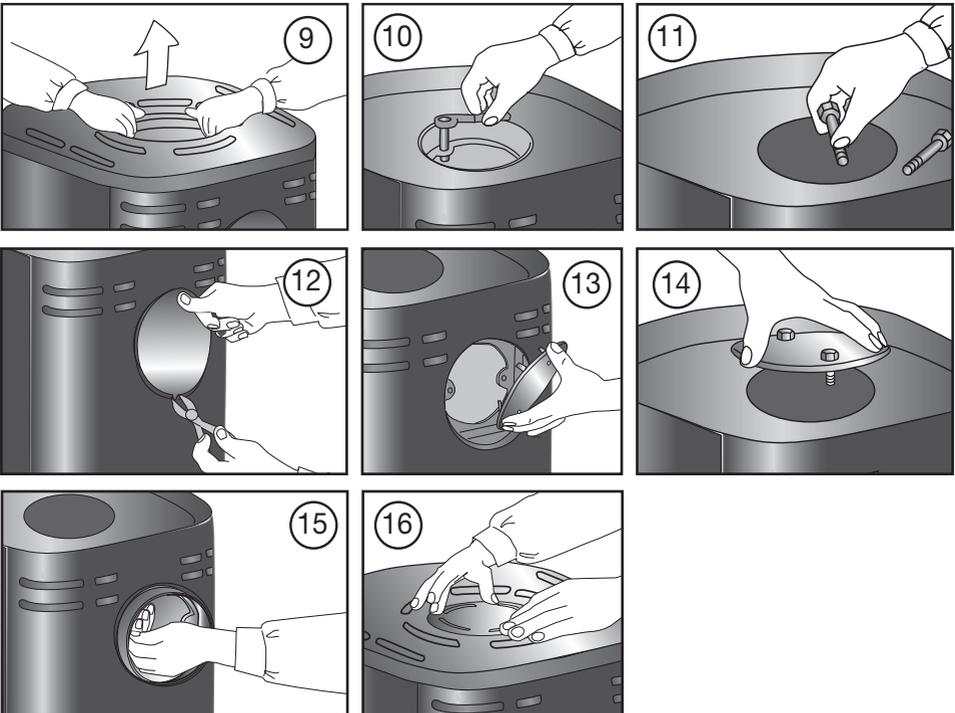
**Cleaning after sweeping the chimney and replacing the stones. Fig 17-23 - Scan-Line 800 standard**
