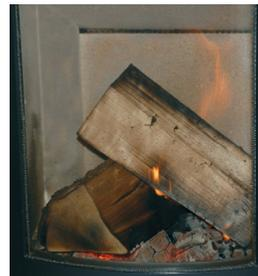
6. Place 2/3 logs on the ash bed ensuring that the wood is not stacked too closely and with the adjust the side airslider to fully on position. The wood will light in 2/3 minutes. Adjust the air slider for optimum combustion.
