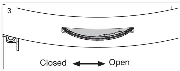
exempt for use in smoke control areas throughout the UK when burning dry wood logs. To comply, a permanent stop is fitted to ensure that the air control slider cannot be closed beyond 35% of its fully open position. A permanent amount of air will therefore enter the firebox to feed the fire producing negligible amounts of smoke and unburnt hydrocarbons. The appliances will only be considered as an exempt appliance if this stop is in place.
