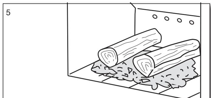
fire once again. Leave the air control fully open and allow the fire to build before refueling with larger pieces of wood. Then adjust the air control for optimum combustion. Do not overload the firebox by loading above the tertiary air diffuser at the back of the firebox and ensure that the wood is retained by the log guard. Always ensure that the wood is not tightly stacked so that air can circulate freely.
