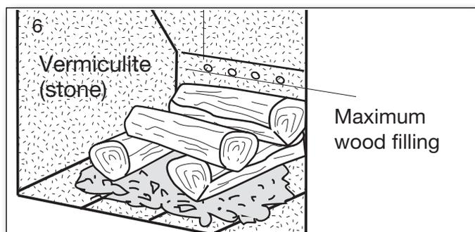
series of air holes and within the outer vent in each side. Fig. 6
